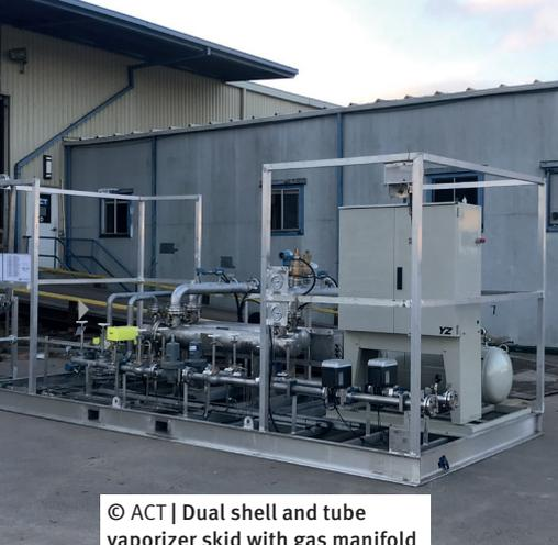
© ACT | Dual shell and tube vaporizer skid with gas manifold
